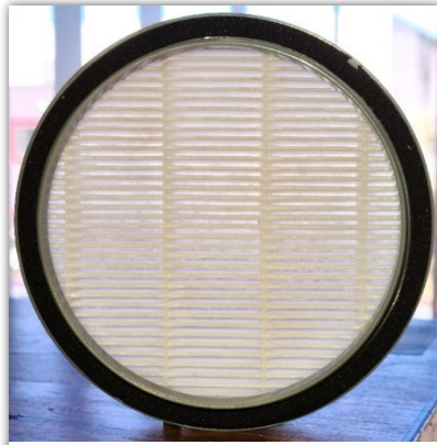
6. Leave the filter to dry for up to 5 days. The filter should pass light when clean.
