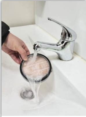
5. Rinse filter until there are no soap bubbles in the filter pleats or rinse water.
